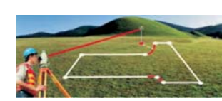
Stake-out pile points with reference to existing structure (P2)
