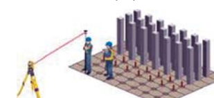
Stake-out pile points with reference to existing structure (P2)
