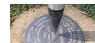
Establishing new benchmarks and cross checking (P3)
